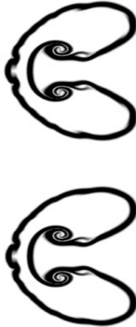
Figure 4. Schlieren image at time t = 511 \mu\text{s} computed with the AMR algorithm (top) and with a fixed grid algorithm (bottom).
